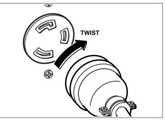
Caution : To connect the appliance to locking receptacle, insert the plug into the receptacle and turn it clockwise to lock.
